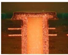
Board Thickness = 120 mils Hole Diameter = 14 mils
